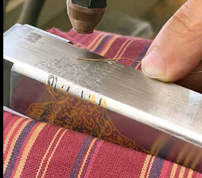
The Gold wire is hammered in the engraving in a cold forging process.
