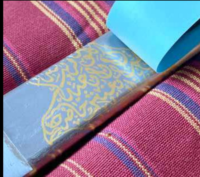
The leveling of the excess Gold Inlay is terminated and final fine honing is under way.
