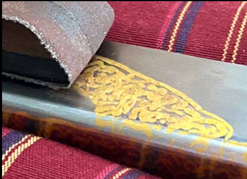
The finished Gold Inlay is overflowing the engraving and requires a long process of sanding down to the steel level.
